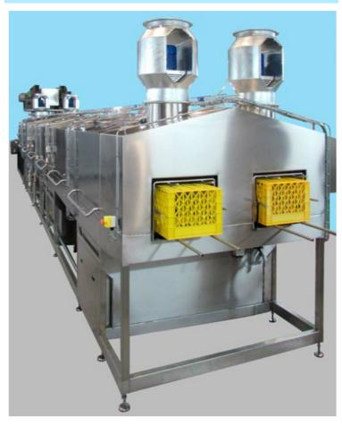
Built at our Brownhills site, the washer, which is 13.5 meters in length, took approximately 20 weeks to build and was designed to wash and dry crates soiled by dairy returns. During their visit to our site to inspect the machine, our client requested further adaptations to meet new requirements from the end user, which Unitech were able to do before shipping the machine in 2 containers to the Middle East.
